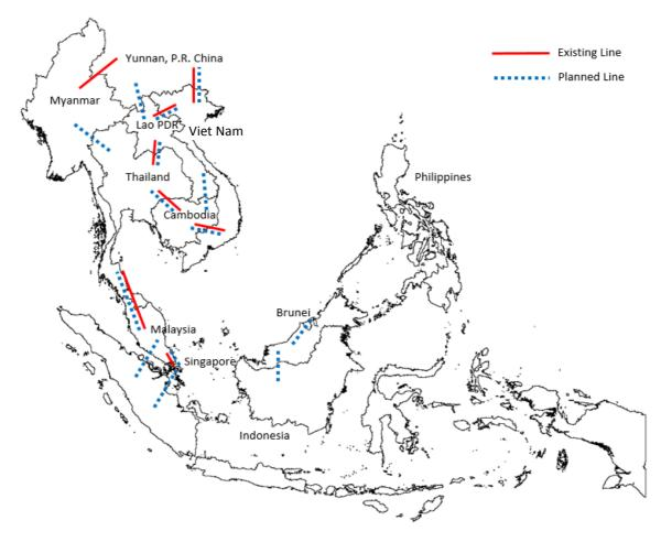
Figure 6.3.3. ASEAN Power Grid Interconnectivity – Existing and Planned
